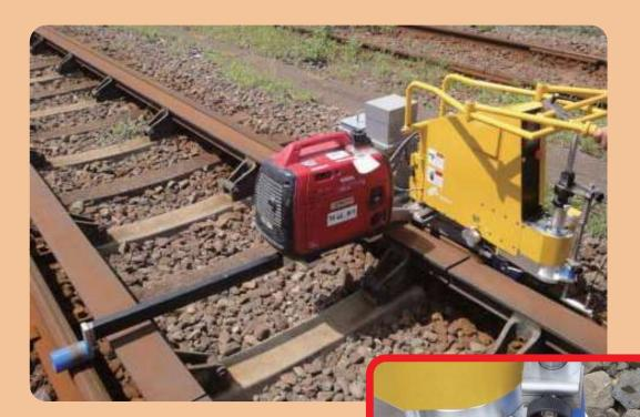
• Automatically fasten-loosen the bolts with off-centering socket to avoid the obstruction
