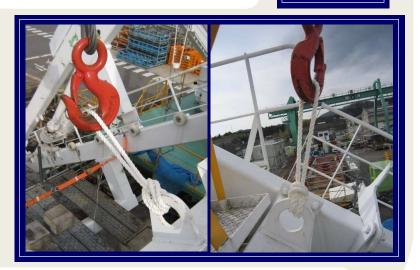
Tie both end rope rings to the eye plates as is shown in the photo. This can avoid loosening or falling of the rope during davit operation.
